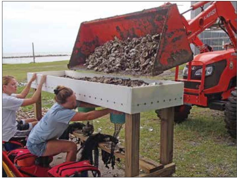
Figure 9. Shell bags being filled at a table designed to aid in filling. Bags are slipped over the PVC pipe affixed to the table; clutch is then loaded onto the top of the table and pushed into the openings, filling the bags.
