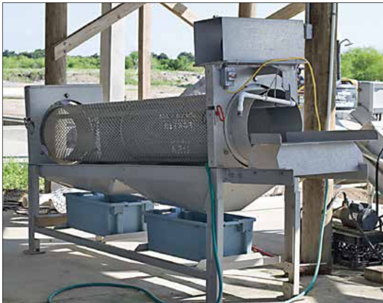
Figure 10. Oyster size grader that can be used to grade and wash seed simultaneously. Seed oysters or clutch materials are loaded into the grader as the drum rotates and water is sprayed into the rotating drum washing shells and allowing oysters/shells to fall through appropriate sized holes in the drum for grading.
