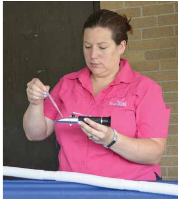
Figure 2. Louisiana Sea Grant agent using a refractometer to test salinity.
