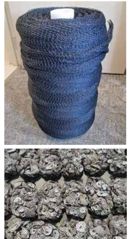
Figure 8. Roll of shell bag material (top) and shellbags cut, filled and ready for handling (bottom).
