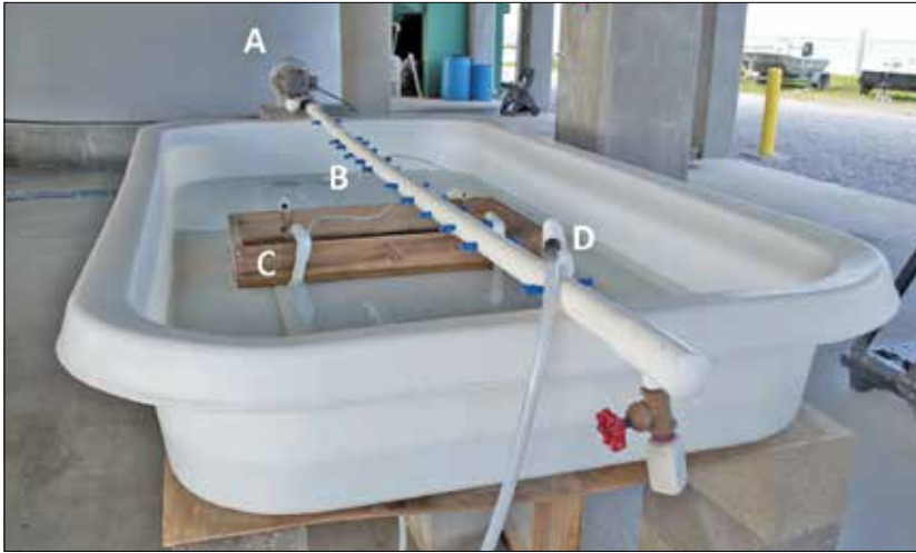
Figure 13. Setting tank. A blower is connected to a manifold that runs along the length of the tank. Flexible rubber tubing connects the manifold to the airlifts attached to setting trays. Water is recirculated from a reservoir by a sump and discharged through a hose positioned at the end opposite the stand-pipe.
