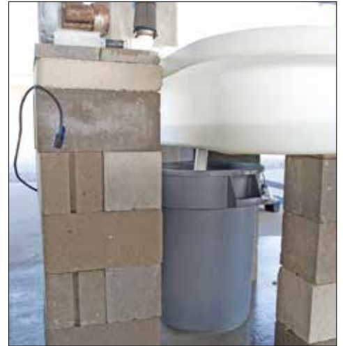
Figure 14. A 35-gallon trash can acts as a reservoir for a setting tank. It is placed under the standpipe drain. Water is then pumped from the reservoir back to the setting tank by a submerged pump and hose.
